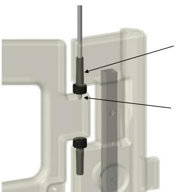
REMOVE THE (4) HINGE PINS AND INSERT INTO THE OTHER SIDE OF THE FRAME – 5/8" HOLES WILL NEED TO BE DRILLED IN THE FRAME KNUCKLES AND 3/8" IN THE DOOR KNUCKLES. CONNECT THE DOOR AND FRAME WITH THE L-ROD.
