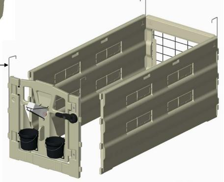
WITH ANY VERSION FRONT - LINE UP THE FINGER TABS OF THE DESIRED PANELS DROP L-ROD THROUGH THE HOLES
