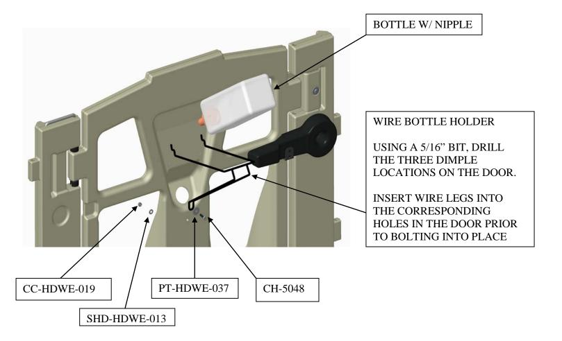
INSTALL THE 1" CAP SCREW (CH-5048) AND THE 1" DIA. WASHER (PT-HDWE-037) THROUGH THE BOTTOM LOOP OF THE WIRE BOTTLE HOLDER.
