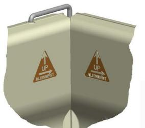
START THE ASSEMBLY BY LINING UP THE TWO UNI-DIRECTIONAL ARROWS IN THE TOP, LEFT, BACK CORNER OF THE FIRST PEN
