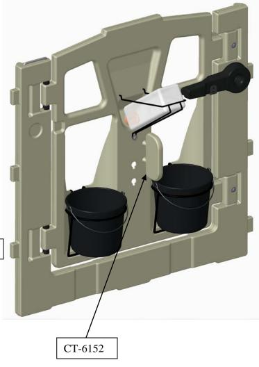
THE (CT-6152) PAIL DIVIDER IS DESIGNED TO BE A TIGHT SNAP FIT.
